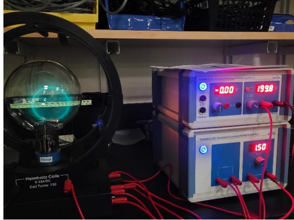
Helmholtz coils without tube to measure magnetic field. Cyclotron orbit with power supplies, V=200V , I= 1.5A
