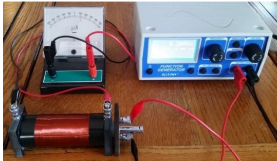
Experiment 3: Solenoid in Solenoid (Quantitative with Function Generator)
