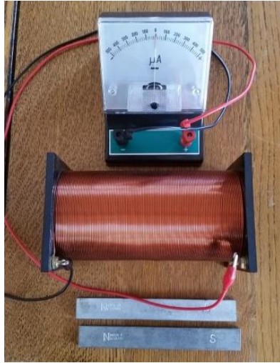
Experiment 1: Magnets in Solenoid (Qualitative). Experiment 2: Solenoid in Solenoid (Qualitative)
