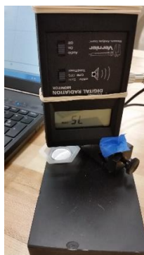
Figure 2, Radiation Monitor ~3 cm above Ba source
