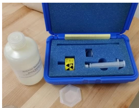
Figure 3, Ba-137 Isogenerator kit and Eluting solution.
