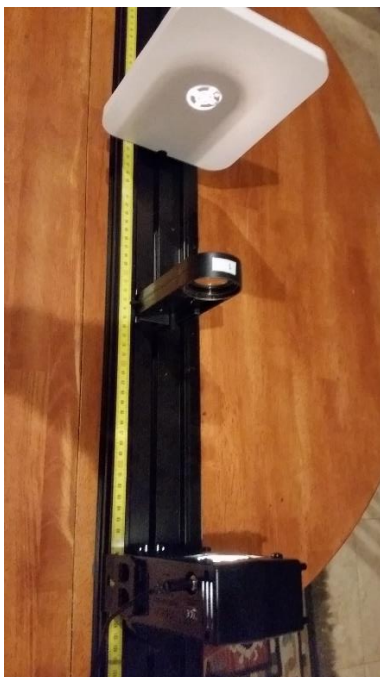
Figure 1, Experiment A Focal Length of a Thin Lens
