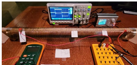
Exciting LC circuit with function generator
