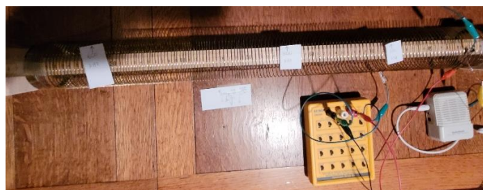
Combining Slinky Inductor, Capacitor and diode to make receiver
