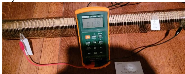
Measuring Inducance between loops on stretched slinky.
