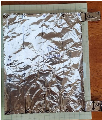
Fig. D1, aluminum foil electrodes separated by Transparency sheet, placed in open notebook.
