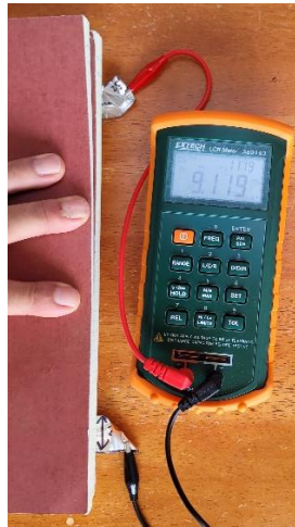
Fig. D2, Measuring capacitance with pressure exerted on capacitor to smooth wrinkles.
