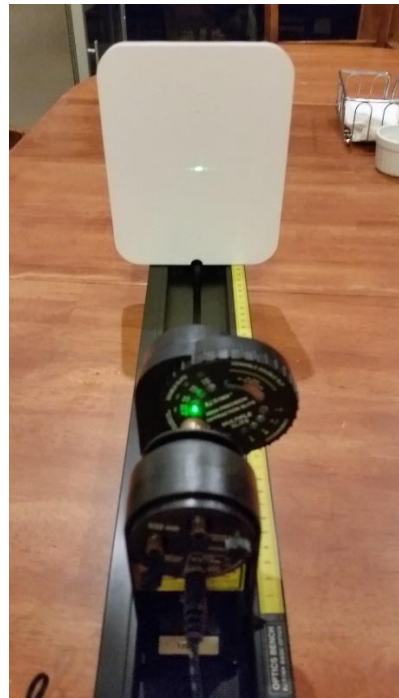
Figure 3, Experiment C Two slit interference, green laser
