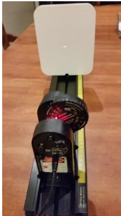
Figure 2, Experiment B Two slit interference, red laser
