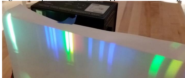
Figure 4, First and Second Order Spectrum from Mercury Lamp
